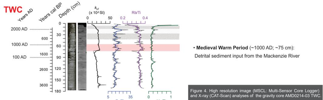
Figure 4. High resolution image (MSCL: Multi-Sensor Core Logger) and X-ray (CAT-Scan) analyses of the gravity core AMD0214-03 TWC.
