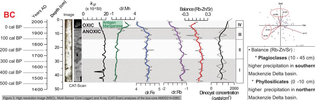
Figure 3. High resolution image (MSCL: Multi-Sensor Core Logger) and X-ray (CAT-Scan) analyses of the box-core AMD0214-03BC.
